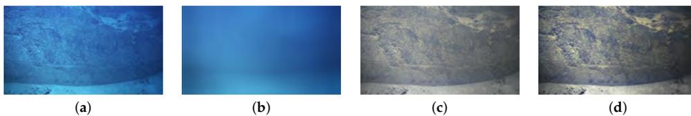
Figure 2. (a) Original underwater (UW) image. (b) Chromatic components ( $\alpha, \beta$ ) of the estimated local illuminant. (c) White balanced image. (d) Final enhanced image.
