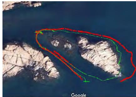
**Figure 20.** Vehicle's trajectory (green) calculated by its dead reckoning system and the camera's trajectory (red) estimated by the SfM, both overlapping a satellite image of the test scenario.
