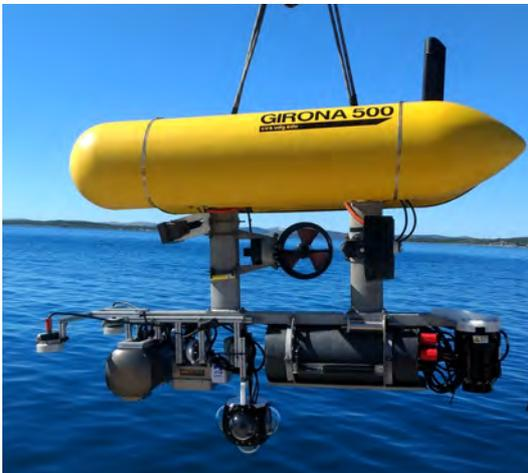
**Figure 6.33:** Girona 500 AUV with omnidirectional and stereo camera system.
