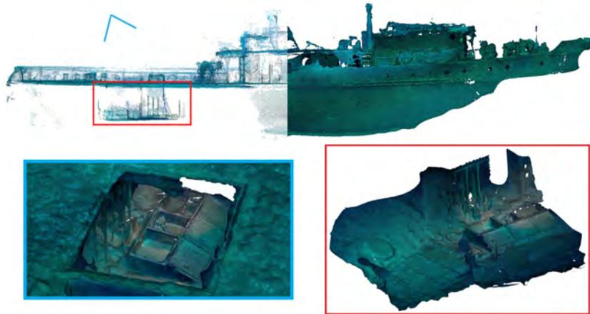
**Figure 6.23:** Side view of a fused dense/textured 3D model of the *Boreas* shipwreck with highlighted successfully reconstructed cargo hold area.
