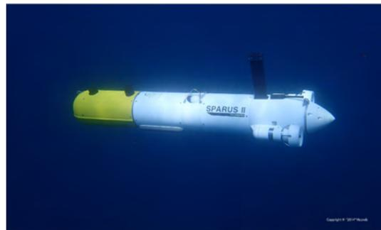
Figure 1. Sparus II, a torpedo-shaped AUV.
