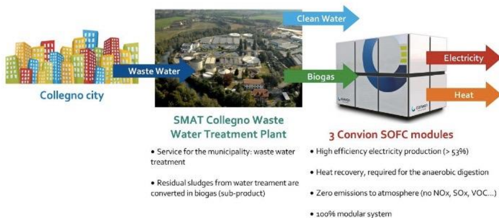
Fig. 22. Waste-to-Energy production system at SMAT's WWTP (DEMOSOFC)
