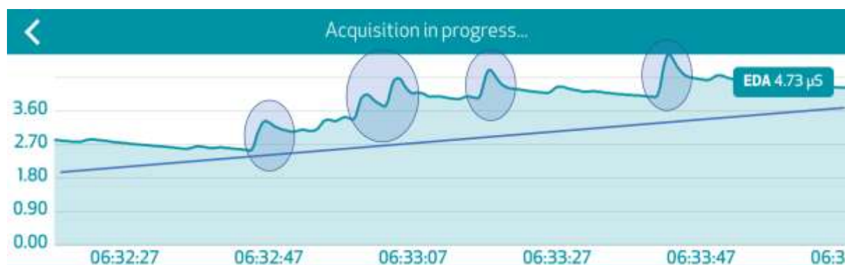
Figure 38: Phasic signals (Circled) over a tonic baseline (Line). Not all of the peaks are stimulus-driven. Source: (Empatica, 2020)
