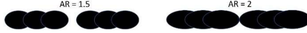
Figure 52: Printing 3 black dots, one white dot, and 3 black dots with AR = 1.5 (left) and with AR = 2 (right)
