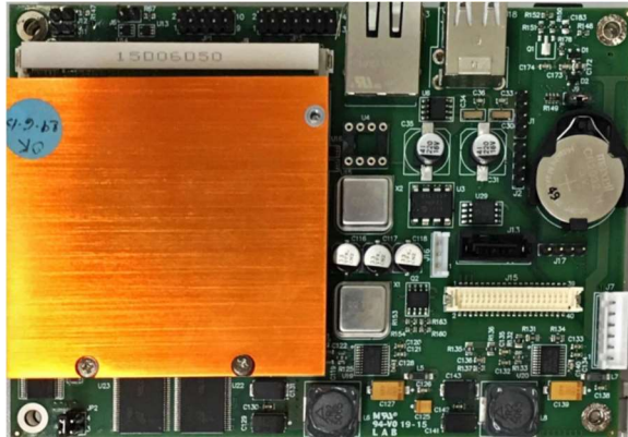
Figure 7: Embedded system and scanning card based on Q7 standard module and customized motherboard used in Macsa's laser marking systems
