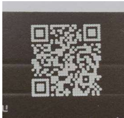
Figure 63: The same sample printed with a short pulse width (40 \mu s) and high laser power (240W).
