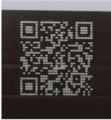
Figure 64: Sample printed with a long pulse width (60 \mu s) and low laser power (60W).
