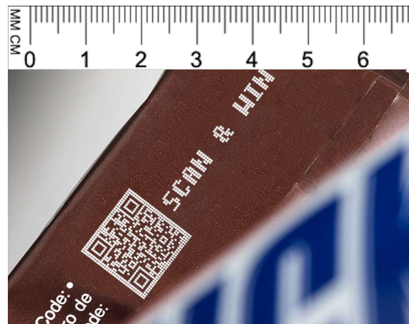
Figure 75: Example of marking with HP f-LDA laser system for very-high-speed (10 m/s) coding applications
