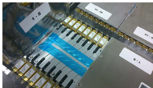
Figure 49: Detail of the f-LDA prototype with diode stacks and fiber umbilical cables
