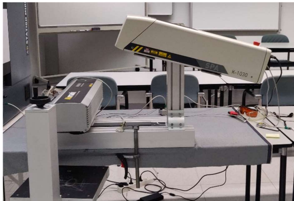
Figure 44: Testing setup containing a CO 2 laser (right) and a UV laser (left).
