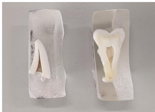
Figure 20. Image of a bovine (left) and a human (right) dental specimen prepared for specular reflectance synchrotron radiation-based Fourier transform infrared microscopy.
