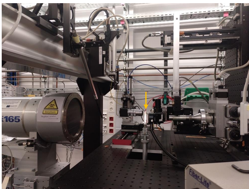
Figure 19. Dental specimen (arrow) ready to be analyzed by tts- \mu XRD in the experimental hutch at MSPD beamline of ALBA Synchrotron.
