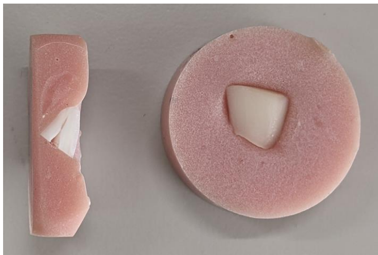
Figure 16. Image of bovine dental specimens prepared for lateral (left) and surface (right) SEM-EDX analysis.
