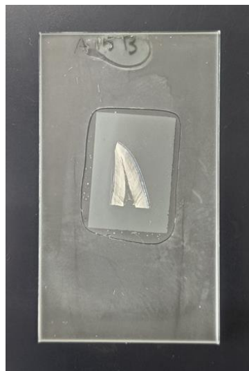
Figure 18. Image of a bovine dental specimen prepared for synchrotron through-the-substrate micro X-ray diffraction.
