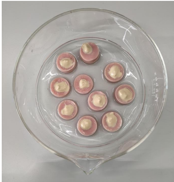
Figure 15. Bovine teeth with NMTD treatment in the vessel before sealing.
