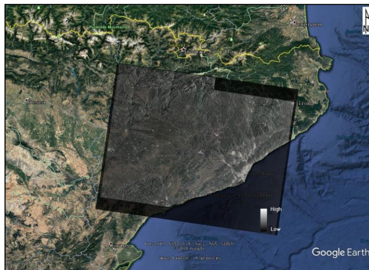
Figure 4.8 Footprint of the processed amplitude image and area of interest. The area is covered by 2 sub-swaths and 7 bursts
