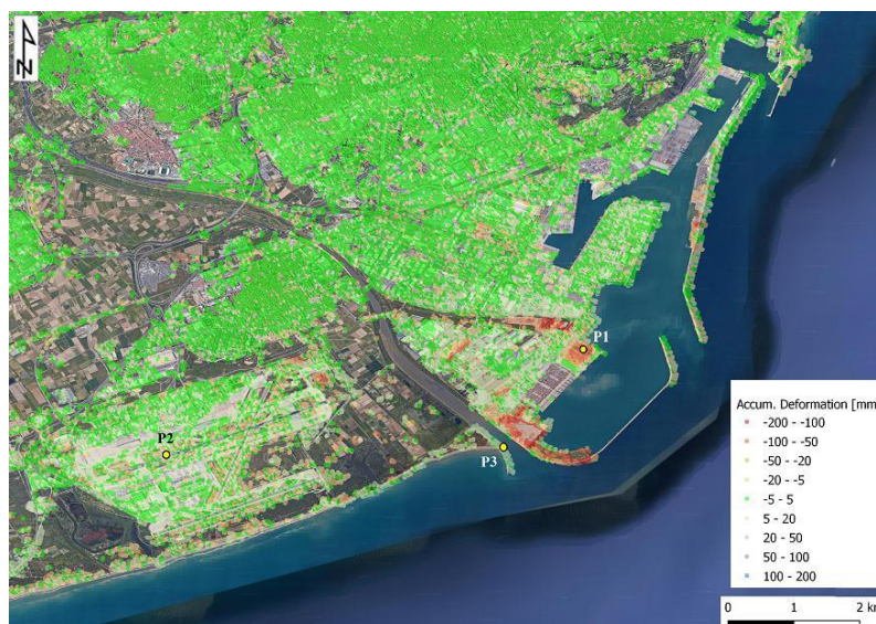
Figure 4.12 Active deformation map of area B (Barcelona Ports). P1 and P2 have notable settlement (between -2 and -6 cm) due to surface loading during the observation period, P3 has a lifting deformation (over 5 cm) caused by the sedimentation.
