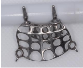
Figure 9. Grade 5 titanium mesh used in this study.
