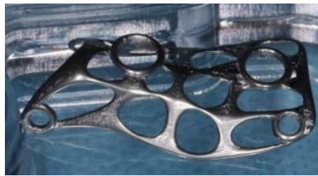
Figure 12: Ti6Al4V mesh used in this study
