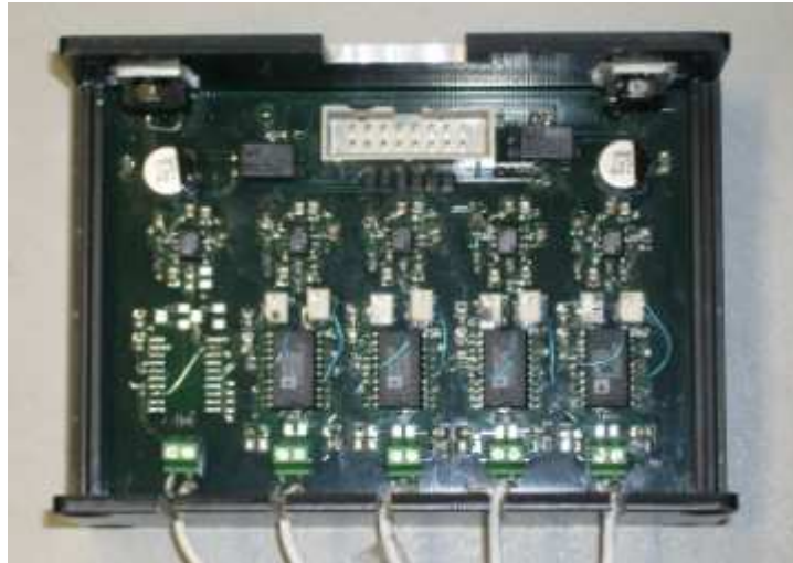
Figure 12: Analog pre-amplifier, featuring an instrumentation amplifier and a low-pass filter for each channel. The board is placed inside of a metallic box to reduce external interferences.
