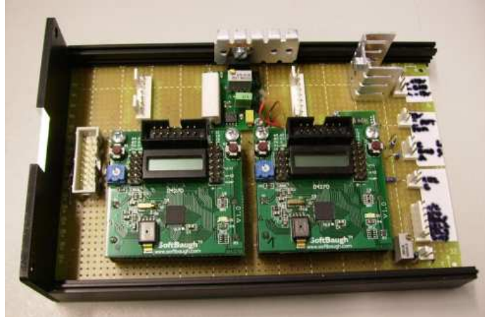
Figure 13: Board featuring both microcontrollers for lock-in routines.
