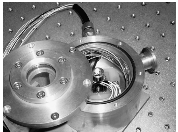
Fig. 6. Vacuum chamber, with a bushing wall to measure thermopile output voltage from outside, and a calcium fluoride window.
