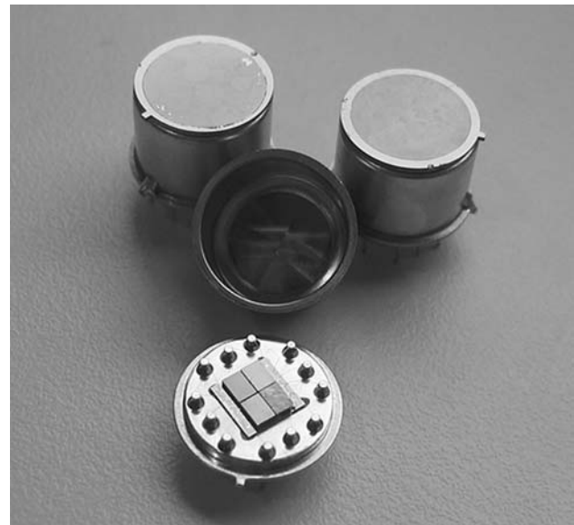
Fig. 8 Completed detectors with the AR coated silicon Fresnel lenses. The open package shows the thermopile array covered by the four narrow bandpass filters and the facing down Fresnel lenses attached to the package lid
