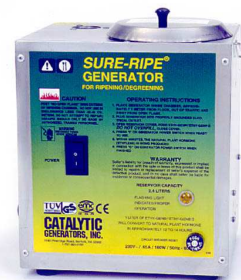
Figure 3: Ethylene concentration can be increased or reduced in today's apple store houses. Right: Catalytic generator to produce ethylene in store-houses (Sure-Ripe Generator, Catalytic Generators LLC, USA). Left: Typical ethylene scrubber bloc diagram. The room air comes in the scrubber, flows through a catalytic layer which is kept hot, cools down while passing through a ceramic heat exchanger, and comes back into the room free of ethylene. (Adapted from Absoger webpage)
