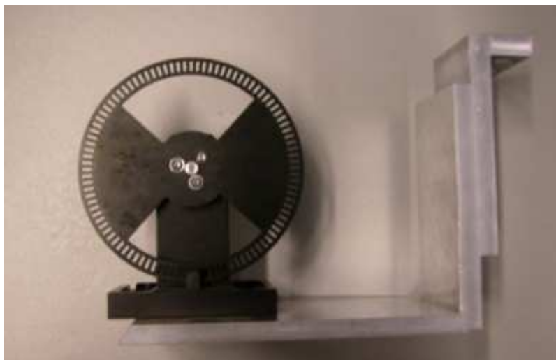
Figure 5: Slot blade for modulating the IR beam. 10.5cm diameter.
