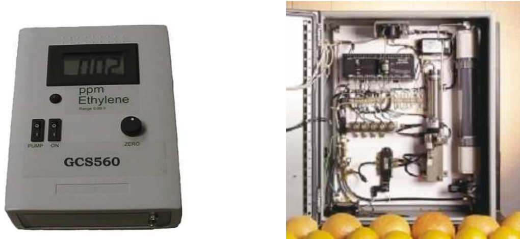
Figure 4: Commercial systems to measure ethylene. Left: Electrochemical based sensor: GCS560 (Storage Control Systems Inc.). Right: Chemiluminescent based sensor: Ethylene Monitoring and Control System (Geo-centers Inc)
