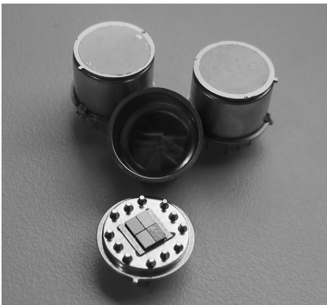
Fig. 12. FL-array, properly aligned and attached to the detector lid of a TO8 package.
