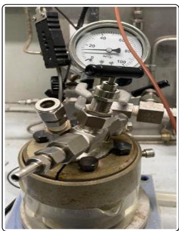
Figure 11: Reactor employed for the cycloaddition of CO 2 reaction.
