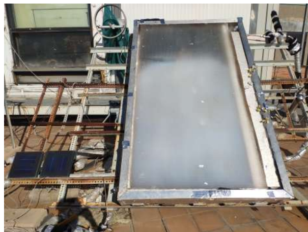
Figure 7.4: Solar collector first version with TIM and aerogel
