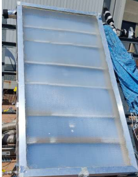
Figure 7.6: Solar collector with fixed aerogel in the test
