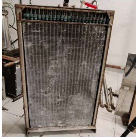
Figure 1.11: Vertical falling film type absorber in [20]
