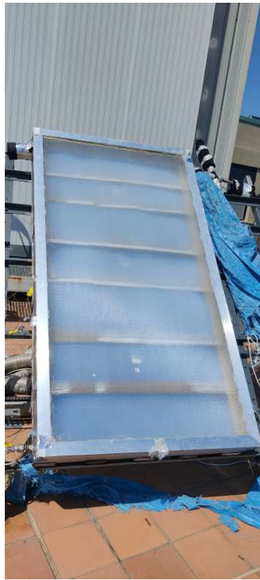
Figure 1.14: A FPC collector with TIM and aerogel of previous work [23], [24]
