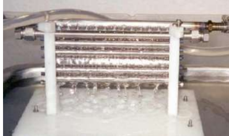
Figure 1.7: Flow pattern of a horizontal falling film over tube bundle in Castro [19]
