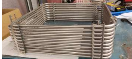
Figure 1.9: Heat exchanger for liquid-liquid SS serpentine in [20]
