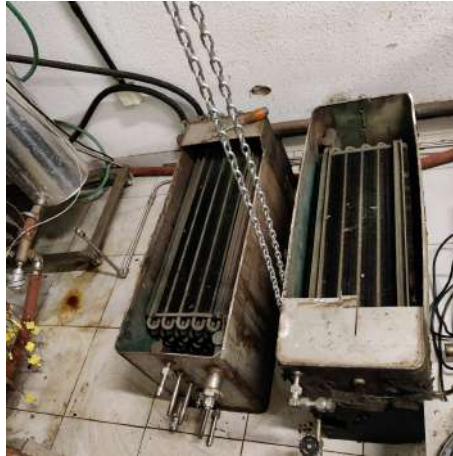
Figure 1.12: A pool boiling type of evaporator in [20]
