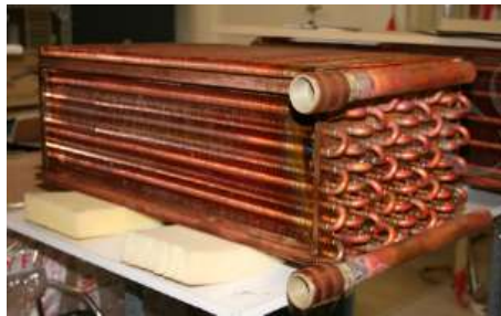
Figure 1.13: Heat exchanger for liquid-liquid copper finned serpentine before installation in Figure 1.12
