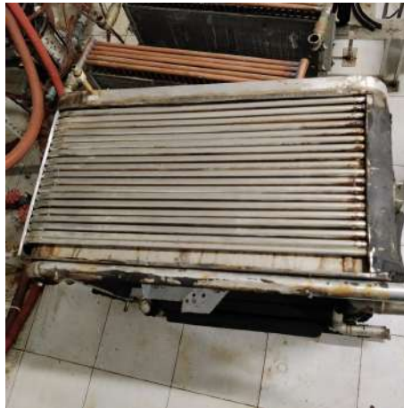
Figure 1.8: A horizontal falling film type generator for a 10 kW absorption machine in [20]
