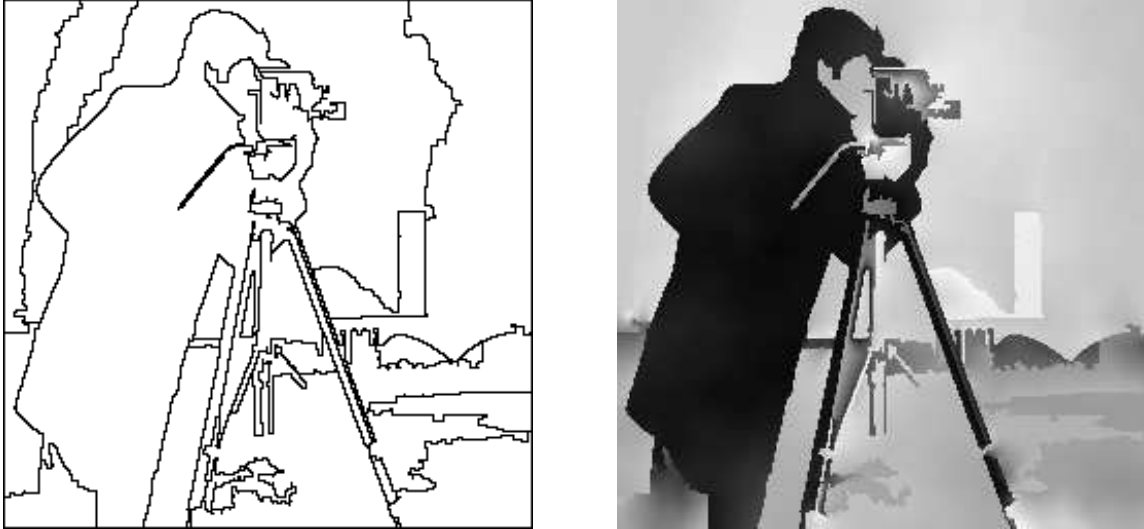
Figure 6.7: Partition of the cameraman image (31 regions) and strong edge component interpolated from ‘region brims’ (0.15 bpp)
