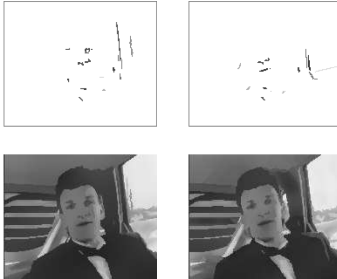
Figure 4.9: Some selected details (top) included in the coded segmentation shown in the first row of Fig. 4.8 result in a subjectively improved reconstruction at 25.2 kbit/s (bottom)
