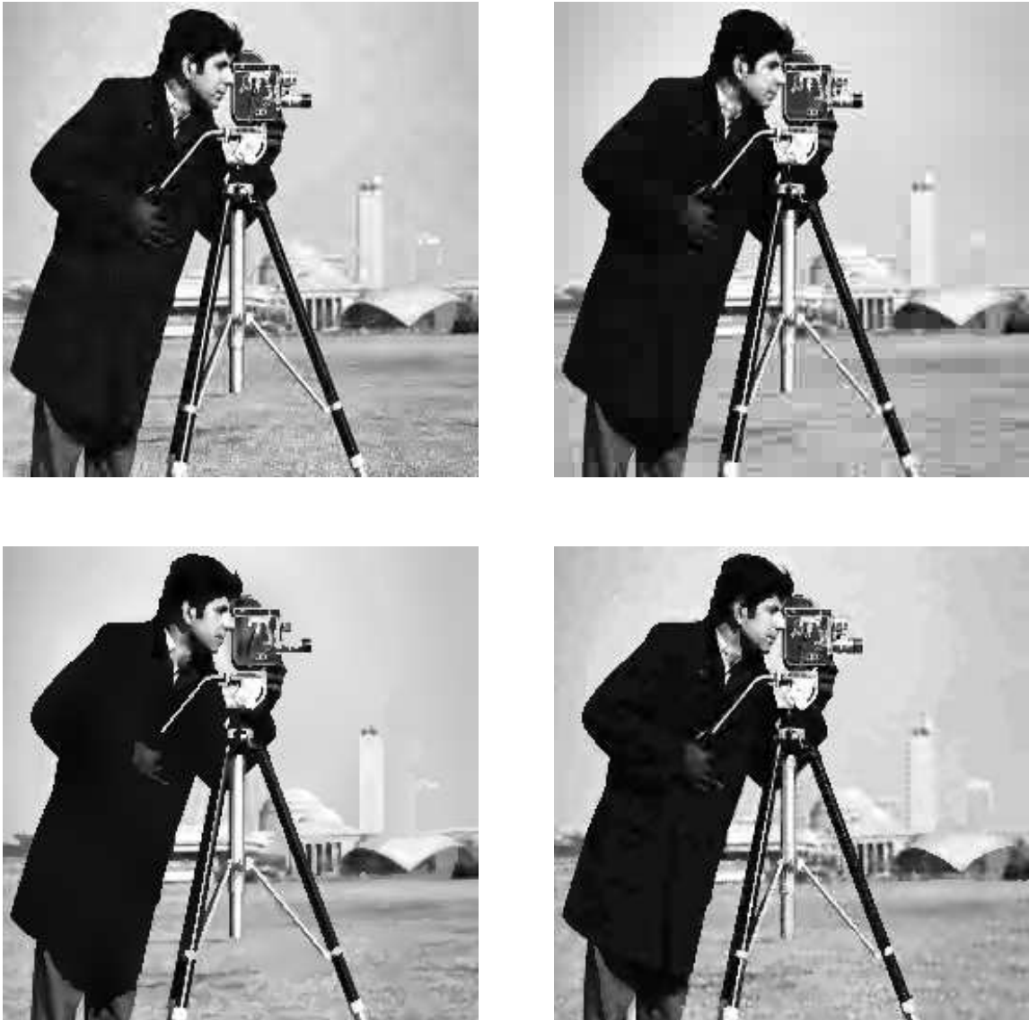
Figure 5.16: Performance comparison at 0.5 bpp: region-based subband coding (upper left), shape-adaptive DCT (upper right), region-based DCT (lower left) and region-based discrete wavelet transform (lower right)
