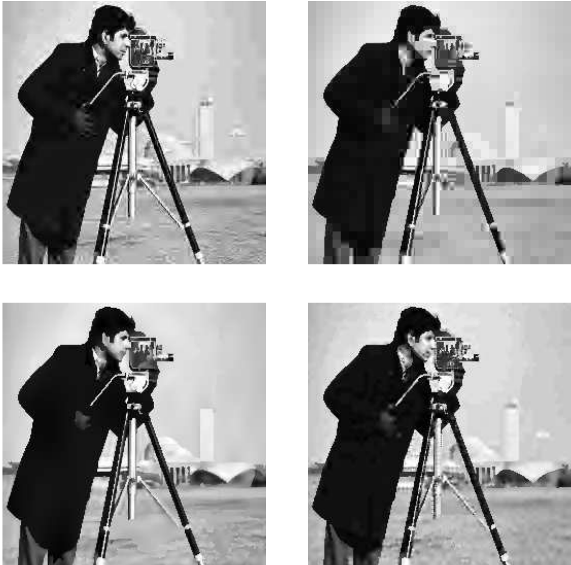
Figure 5.17: Performance comparison at 0.35 bpp: region-based subband coding (upper left), shape-adaptive DCT (upper right), region-based DCT (lower left) and region-based discrete wavelet transform (lower right)
