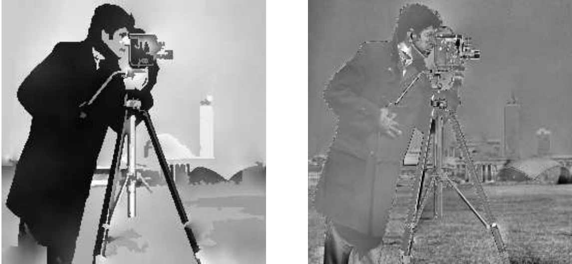
Figure 6.10: Two-component coding (strong edges + details) of the cameraman image at 0.18 bpp and coding residue
