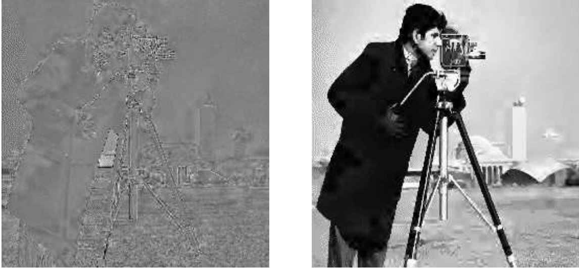
Figure 6.11: Subband coded textures at 0.15 bpp and three-component coding (strong edges + details + texture) at 0.33 bpp
