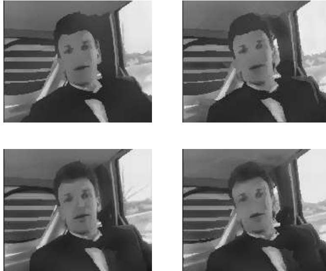
Figure 4.8: Two coded frames of the sequence car-phone at 21 Kbit/s (top row) and 40 Kbit/s (bottom row)
