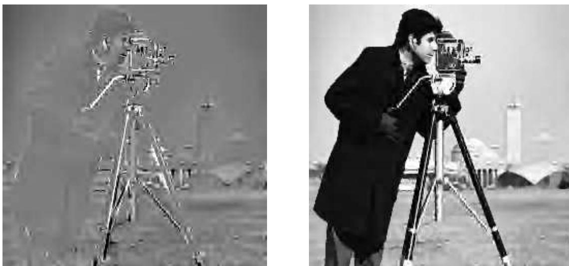
Figure 6.4: Subband coding of the texture component (0.15 bpp) and two-component reconstruction at 0.32 bpp
