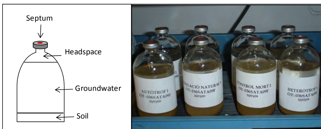
Figure 3.4. Schematic diagram and picture of microcosm tests performed in set 1.
