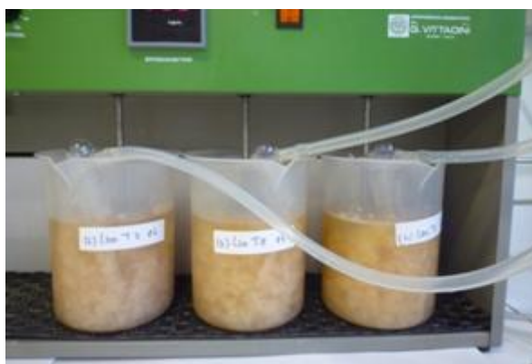
Figure 2-5. Laccase–TEMPO treatments conducted in the jar testing apparatus.
