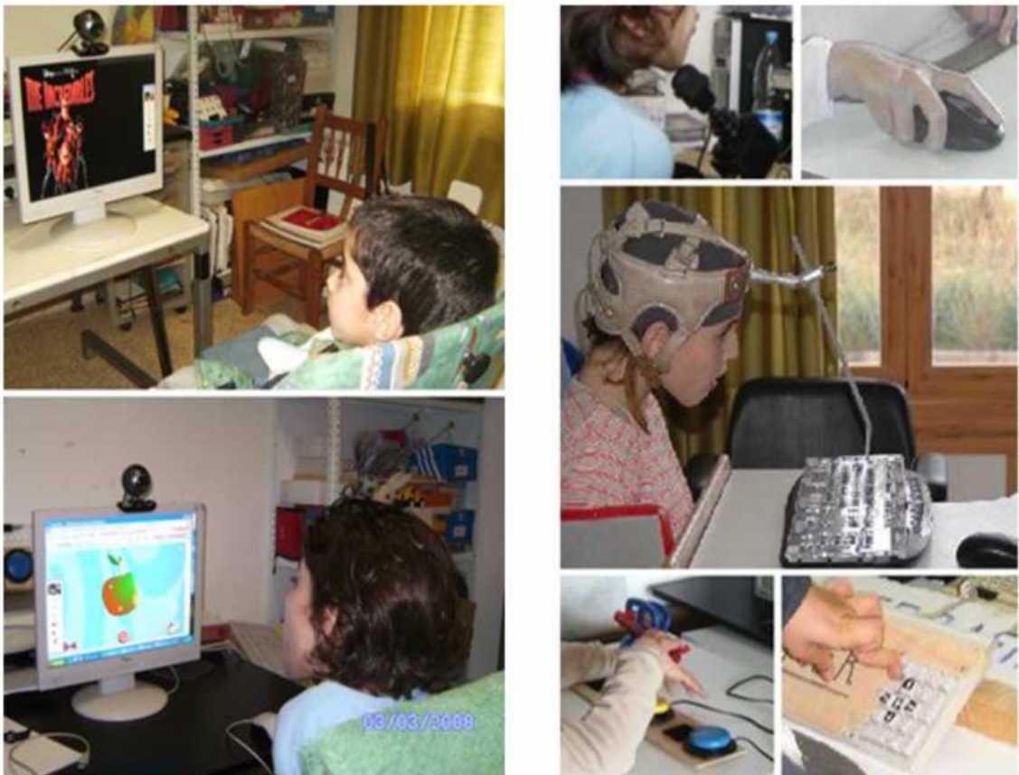
Figure 4.1: In the left column users are working with the hands-free interface. In the right column several other assistive tools which are also used: joystick held with the chin, mouse, head wand, switches and numerical keyboard.
