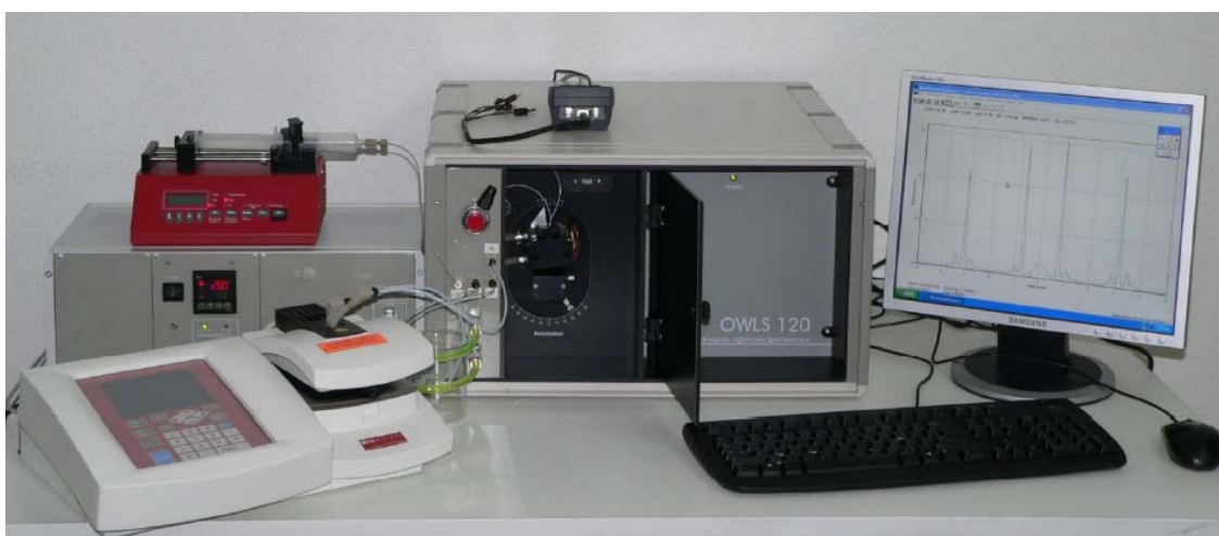
Figure 1.15.- Commercial set-up of the OWLS system (Microvacuum Ltd., Hungary)
