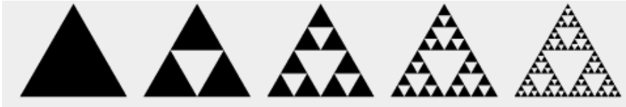
Figure 2.4: Construction of the Sierpinski gasket. Starting from a filled triangle, remove from the middle a triangle whose area is one fourth of the total. In the next step, we repeat the same procedure for the remaining three filled triangles, and this process is iterated indefinitely.
