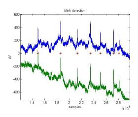
**Fig. 8** EOG sample recorded by ENOBIO. The blue and green lines correspond to FP1 and FP2 respectively. The Red crosses mark the position in the signal where a blink is automatically detected by our algorithm.
