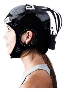
Figure 5.5: Side view of the ENOBIO sensor in its EEG cap configuration
