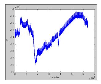
Figure 3.6: Sample of ECG raw data captured with ENOBIO. We can see typical low frequency drifts in the signal. We can also observe a high frequency drift around sample  $0.5 * 10^4$ . The ENOBIO sampling rate is 250 Hz
