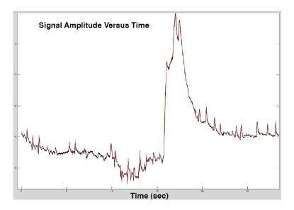
Figure 3.3: Red line is the artefact estimation computed by the algorithm that will be subtracted to the raw signal (black line)
