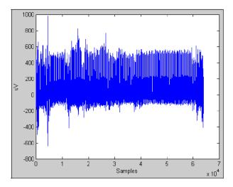
Figure 3.8: First ECG artefact removal. Notice that all the points higher than 1000  $\mu$ V or lower than -1000  $\mu$ V are removed
