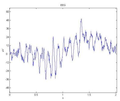
**Fig. 1.2** ENOBIO EEG recording sample of 2 seconds with no pre-processing. The alpha wave (10 Hz characteristic EEG wave) can be seen.
