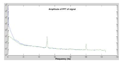
Figure 3.4: Spectrum before (blue) and after (green) applying the artefact corrector
