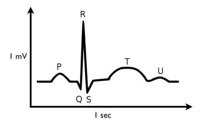
Figure 1.3: Elements of the ECG-complex
