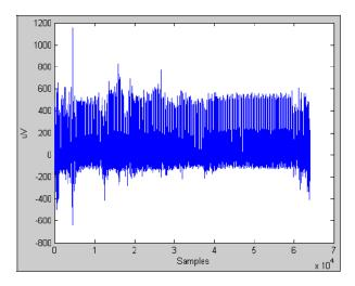
Figure 3.7: Band filtered ECG signal. We can see that the high frequency drift present in fig. 3.6 around sample  $0.5 * 10^4$  appears now as a strong peak. The ENOBIO sampling rate is 250 Hz
