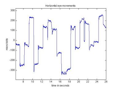
Figure 1.4: Sample of an EOG recording with the ENOBIO sensor. The electrodes were placed horizontally in the corner of the eyes and thus the horizontal movement of the eyes can be observed
