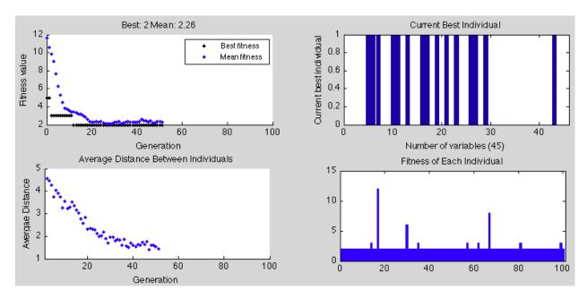
Figure 4.13: Example of the evolution of the Genetic Algorithm applied for feature selection
