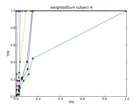
Fig. 7. Example of the extensive search procedure in the parameterization of the weighted sum operator for fusing subject 4 EEG and ECG modalities. Not all parameter results are shown for the sake of clarity. The ROCs (color coded) and its corresponding AUCs are computed on the fusion result. The parameters deliver several ROCs from optimal (red) to worst (green).
