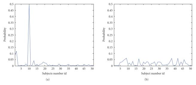
FIGURE 1: PDF for normal situation for subject 10 (a) and for intruder situation (b). In (a), notice that if a probability threshold is set to 0.15, subject 10 will be authenticate only if he claims to be subject 10. In (a), the intruder would not be authenticated in any case.
