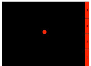
Screenshot of the BCI based biometric system. The 4 targets in the left represent the numbers 1, 2, 3 and 4. The subject has to hit those targets in order to input his/her password. The ball has a constant x-speed. The subject controls the vertical movement of the ball by performing mental imagery movements.
