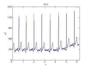
Fig. 7 ENOBIO ECG recording sample of approximately 6 seconds with no pre-processing..
