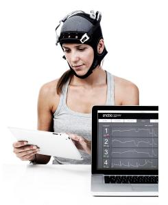
Figure 5.6: Frontal view of the ENOBIO sensor. The data acquisition software can also be seen
