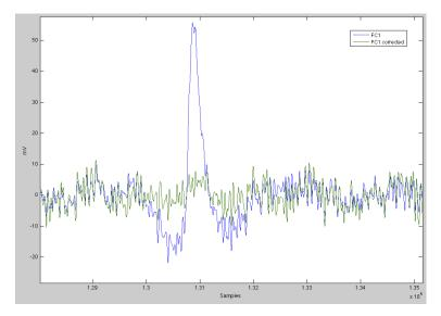
Figure 4.2: FC1 channel corrected from EOG artefacts vs raw FC1 channel. Sampling rate = 1024 Hz
