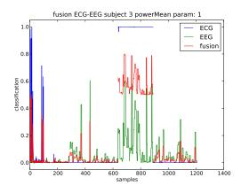
Fig. 8. Example of the compensatory behavior of the power mean operator on subject 3 classification scores (x-axis) when being optimally parameterized. True Positives, i.e. authentications of subject 3, are placed in the samples around the interval [650, 900]. The remaining ones correspond to results of impostor tests. In this case the power mean operator decreases the value on all the samples, but in such a way that TP maintain the maximal value.
