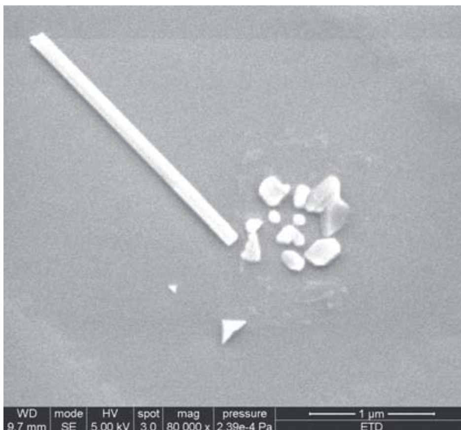
Figure 3-23 Close-up of a high dosage 2x2 array showing variety of nanostructures including nanowire, nanodots in triangular form and irregular shaped form. Array size received 2000 pC and had 750 nm pitch on STO.
