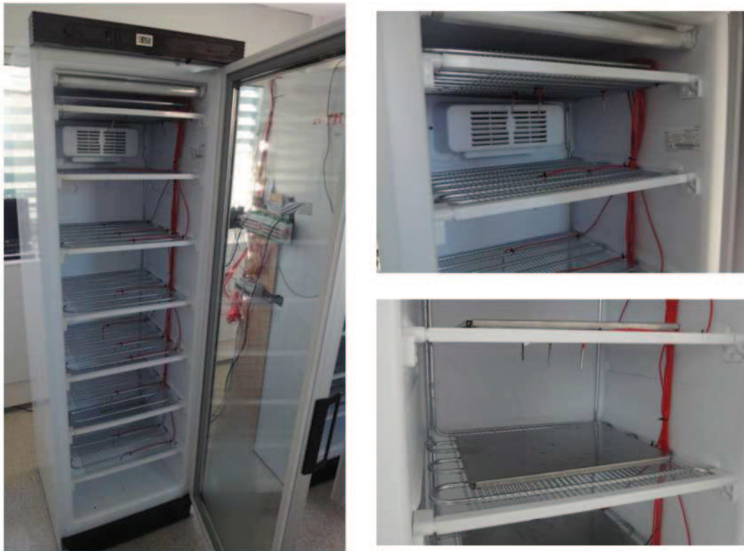
Figure 23. Commercial freezer used in the experimentation and location of the PCM plates.
