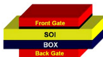
(f) Planar Double-gate on SOI
