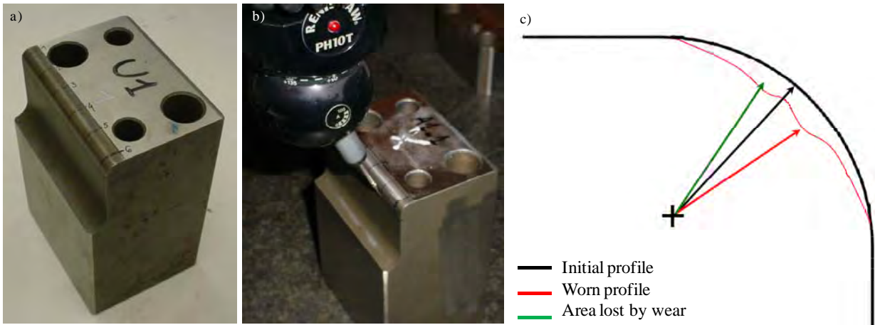
2.5.14 a) - b) Profile measurement at the tool edge; c) schema of the estimation of material lost by wear (tool radius variation)
