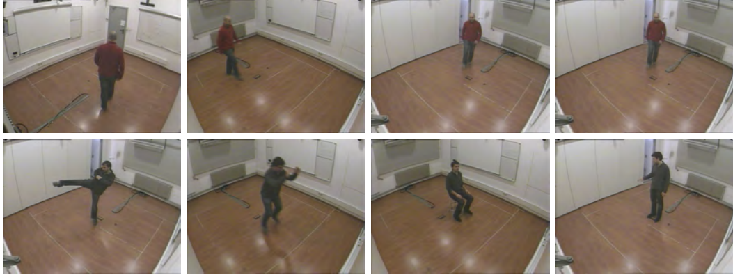
FIGURE 4.27: Multi-view data-set samples. Top row: The four available viewpoints during walk action. Bottom row: Kick, jump, sit and bounce samples.
