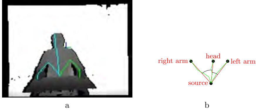
FIGURE B.3: Extrema identification during pose initialization: a) Example of the fork pattern produced by geodesic paths in the neighborhood of the source point. b) The fork pattern is matched by checking that the cosinus of the angles between paths are in a given interval; then we can identify the three key end-effectors
