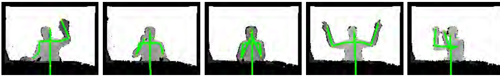
FIGURE B.6: Tracking results in desktop upper-body sequences recorded with Kinect. 256 particles per layer are used.
