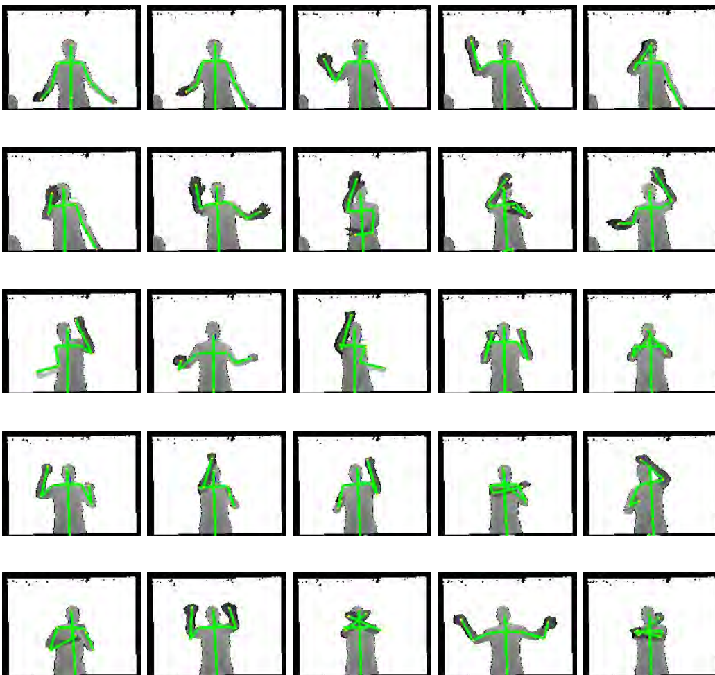
FIGURE B.6: Tracking results in desktop upper-body sequences recorded with Kinect. 256 particles per layer are used.
