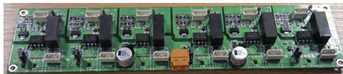
Figura A.5: Placa Gate drivers
