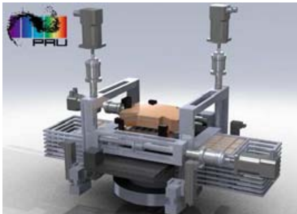
Figure 1.12: Lateral view of the inside of the PAUcam. The top piece is the Copper cold-piece that maintains the CCDs at constant and uniform temperature.
