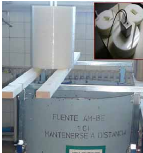
Figure 5.8: Experimental test configuration with Schottky diodes - The polyethylene cylindrical container consists of parallel cylindrical sheets with 20 cm diameter. The ^{241}\text{AmBe} source was fixed at less than 1 cm distance near the container and at the same height as the inner silicon detector. The inset shows the box containing the silicon detector and the front-end electronics inside the aluminium box.
