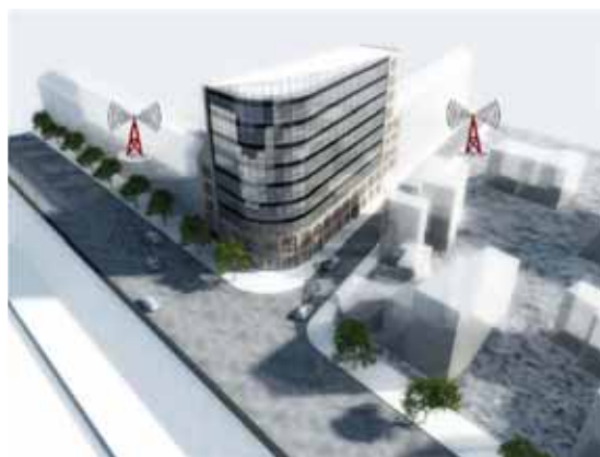
Figure 1.4: Sketch of monitoring tags in REWARD - The monitoring tags of the REWARD system will be installed in law enforcement vehicles or fixed stations and will send their location and measurement data to a central monitoring station if an abnormal situation is detected [21].
