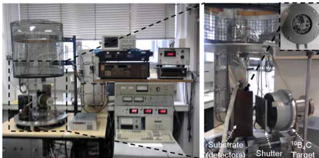
Figure A.16: RF Sputtering machine for PVD - Photographs of the RF sputtering machine used in this work. The detectors were placed within the substrate holder, which is positioned in front of the ^{10}\text{B}_4\text{C} target.
