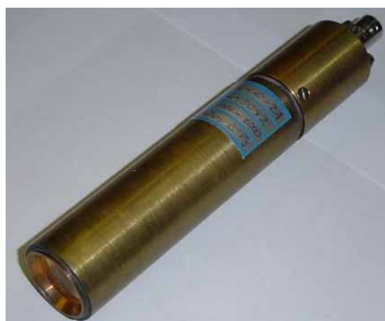
Figure 2.10: Image of a typical BF3 tube - Model G-10-2A. Active Length: 60 mm and diameter: 2.54 cm.
