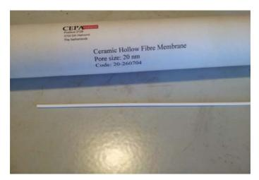
Figure 4-1 Single ceramic hollow fiber membrane
