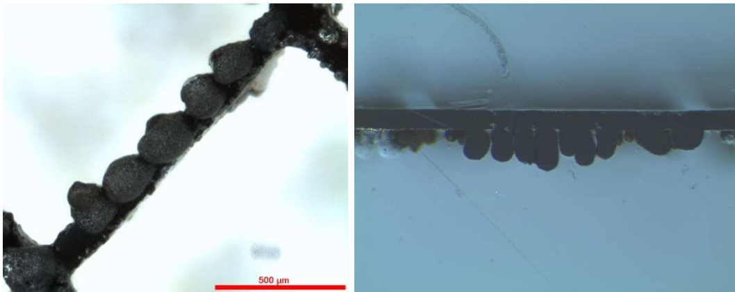
Figure 8. Dross deposition for peak pulse power 300 W, pulse frequency 3000 Hz and cutting speed 250 mm/min sample a) bottom image from optical microscope (50X), b) cut surface image from optical microscope (80X).
