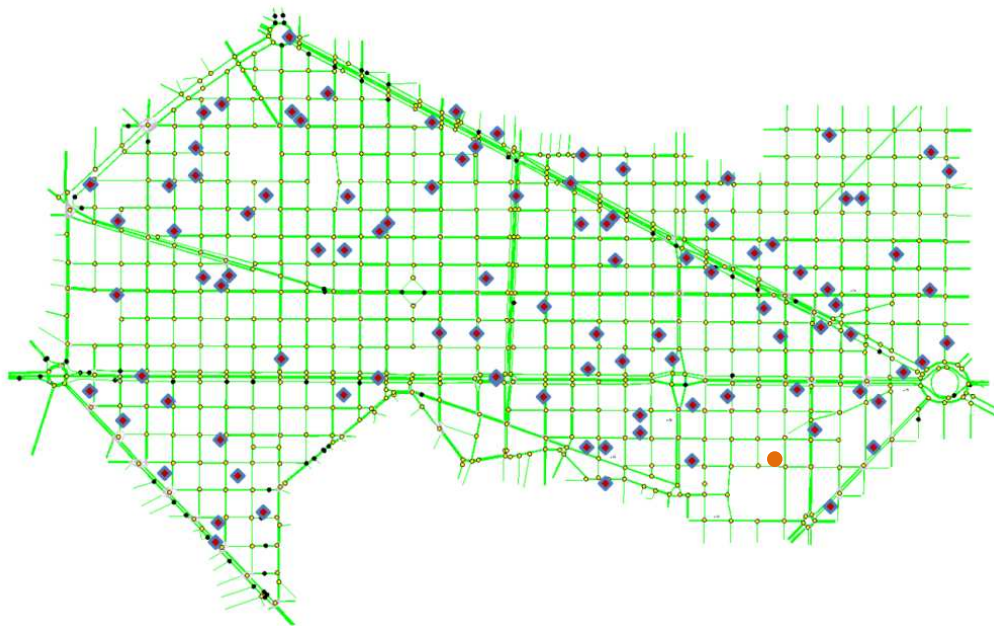
Figure 7.14 Microscopic model of the L'Eixample network
