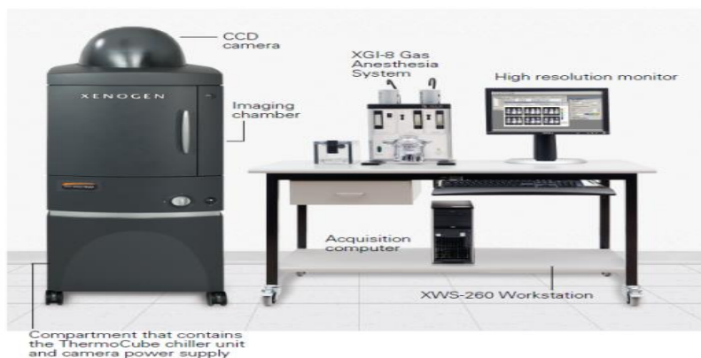
Figure 8.- IVIS Spectrum from Xenogen for In vivo and in vitro optical imaging. Image extracted from IVIS manual.
