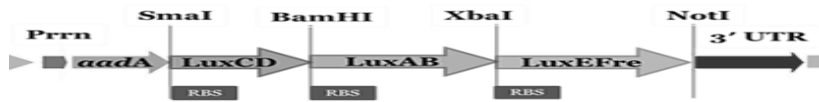
Figure 33.- pLD luxCDABEG expression cassette showing the synthetic restriction sites and RBS upstream every pair of genes.
