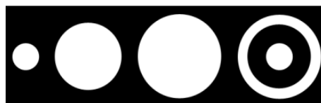
Figure 8.2: Pupils for which optical quality through-focus was predicted. The small aperture pupil of 1.6 mm, a natural photopic pupil of 4 mm, a natural scotopic pupil of 5 mm, and the annulus pupil of 5 mm (inner inlay diameter 1.6 mm, outer inlay diameter 3.8 mm).
