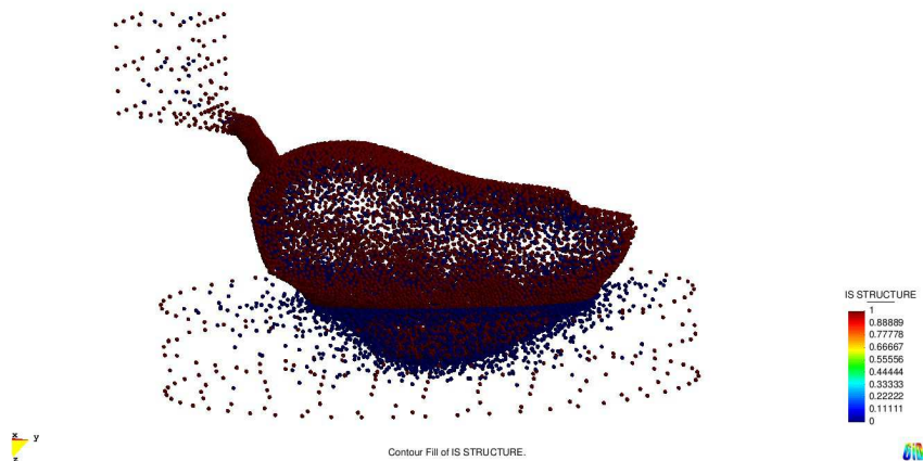
Figure 3.68 – Nodes representing fluid (in blue) and structure (in brown)
