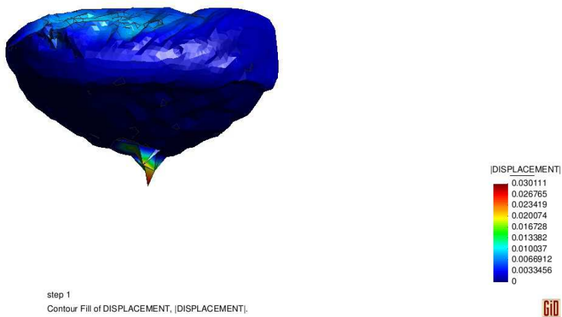
Figure 3.86 – Representation of displacements countours on bladder surface and fluid at time 0.01s (70ml) and time 1.0 sec (63.8ml)
