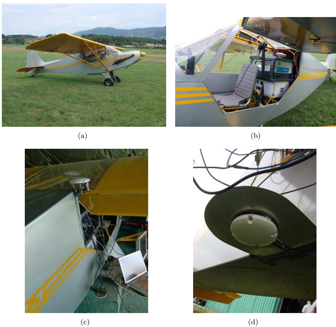
Figure 7.9: GRASS experimental campaign GNSS-R Instrument Installation: (a) General view of the ultralight aircraft. (b) Interior view of the aircraft's cabin with the instrument on-board. (c) Detailed view of the direct and reflected antenna installation. (d) Detailed view of the reflected antenna installation and ground-plane.
