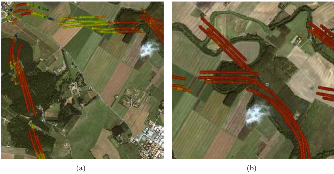
Figure 8.25: Geo-referenced specular points over Google Earth images of the Forcoli Test site. (a) \Gamma'_{rl} and (b) \Gamma'_{rr} apparent reflectivities during Flight 4. The color scale corresponds to the intensity of the reflection coefficients within the range 0.1 (red) up to 0.75 (blue).
