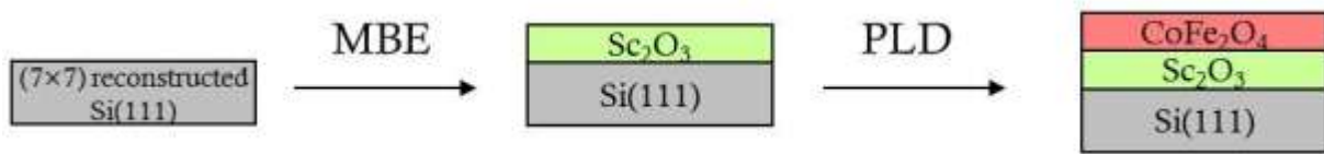
Figure V.4: Sketch of the elaboration of the CFO/ \text{Sc}_2\text{O}_3 films on \text{Si}(111) .
