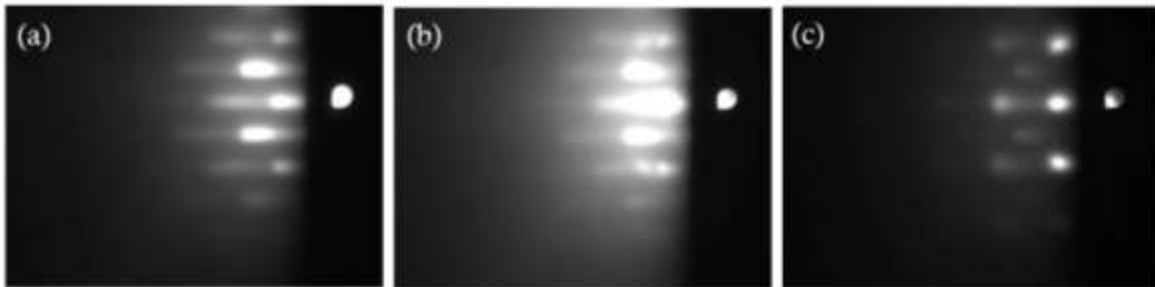
Figure III.7: RHEED patterns taken at 1.2^\circ along [100]_{\text{STO}} : before CFO growth (a), after 40p of CFO deposited under an oxygen partial pressure of 10^{-4} mbar (b), and (c) under 0.1 mbar of oxygen and 250p of CFO.
