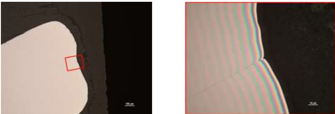
Figure II.13: Picture of the sample prepared by mechanical polishing by tripod to bevel. The glue joint is visible in the zoom, and the fringes attest the transparency to electrons of the sample.
