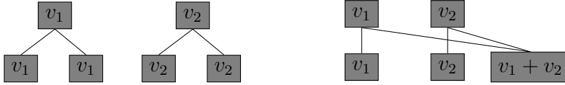
Figure 2.1: Left: a [2, 1, 2] repetition code applied to two coordinates. Right: a [3, 2, 2] parity check code applied to two coordinates.
