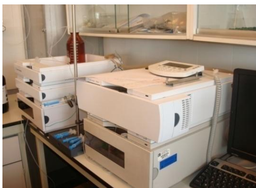
Figure 37. GPC chromatograph used for the molecular weight determination
