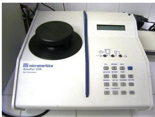
Figure 34. Gas pycnometer employed for the density determination.
