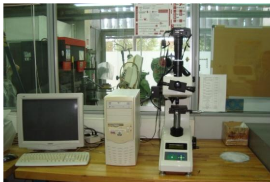
Figure 39. Microhardness tester used for the determination of the Knoop hardness of the prepared thermosets.
