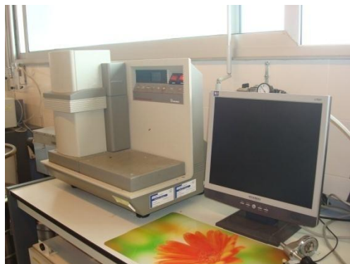
Figure 30. DMTA equipments used to study the viscoelastic properties of the prepared thermosets.
