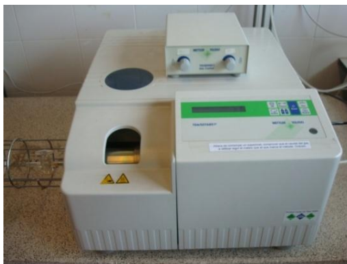
Figure 33. Thermobalance used for the thermal stability evaluation.
