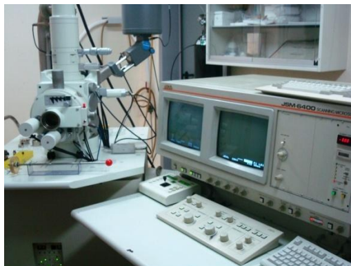
Figure 35. SEM equipment used for obtaining surface images.
