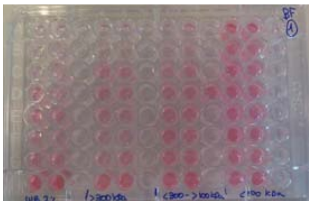
Figure 7.1. Picture of the in vitro biofilm inhibition assay showing the already stained biofilm in the positive control wells (row H). This miniaturized test allows the comparison in a dose-response manner of each sample dilution, in this case corresponding to WB extract, the >300-kDa, <300>100-kDa and <100-kDa fractions.
