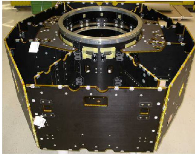
Figure 2.3: General view of the spacecraft. The cylinder in the central part is thought for the LCA placement and the rest of the structure will allocate the remaining subsystems, such as front-end electronics, onboard computers or other units.
