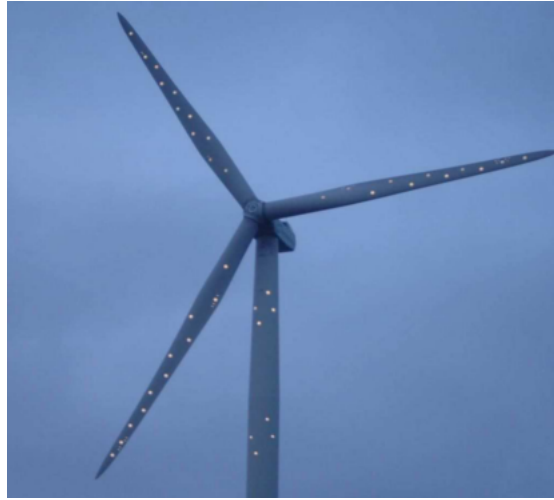
Figure 2.4. The Markers Ozbek [131] used to measure the wind turbine
