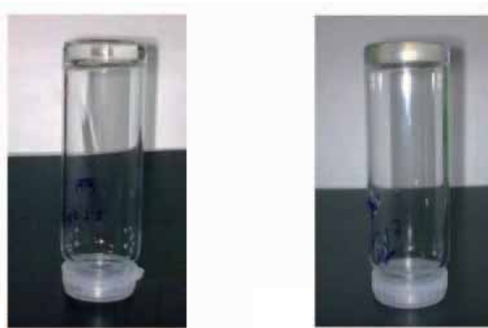
Figure 13. Gels from 40 mM solutions of dipeptides ( S,S,S,S )-6 (left) (1) and ( S,S,S,R )-6 (right) in toluene.
