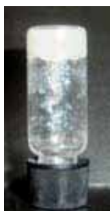
Figure 11. Gel formed from a 1:3 dichloromethane/pentane 5.8 mM solution of the N -Boc protected tetrapeptide 3 .
