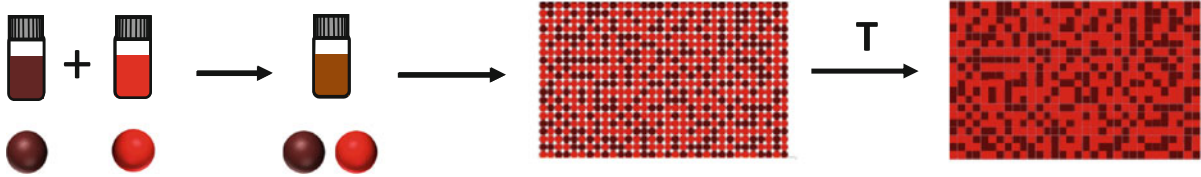
Fig. 2 Scheme of the procedure used to produce binary nanocomposites from solution-processed nanocrystals
