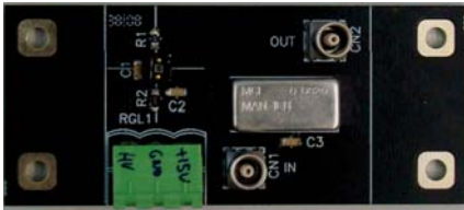
Figure 2.7: SiPM basic test board
