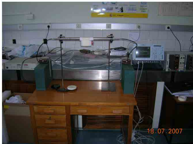
Figure 4.1: Experimental setup. Counter is held by bars. The neutron source is placed inside the polyethylene matrix which is attached to the center of the counter.
