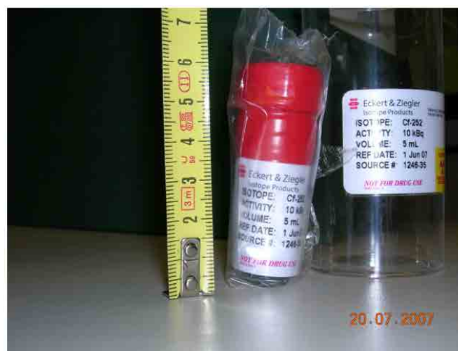
Figure 4.3: Neutron source used in CIEMAT laboratory.
