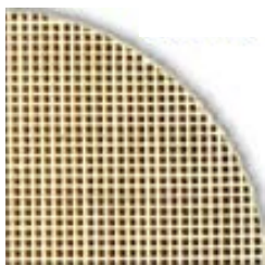
Figure 15. Monolithic catalyst substrates [104] .
