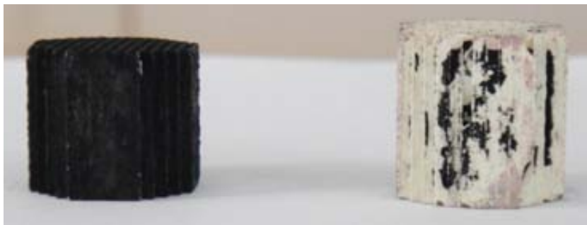
Figure 66. Cordierite monolith after impregnation with a Au(2wt%)/MWCNTs catalyst (left) and after being oxidised at 400 °C in a continuous flow of 100 mL/min (right).
