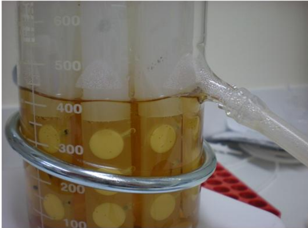
Fig 9 – The CDC Biofilm Reactor, detail: teflon coupons (biofilm growing surfaces) immersed in broth
