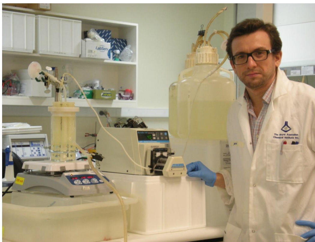
Fig 11 – the doctoral candidate and the in vitro dynamic model for studying the activity of colistin and doripenem against biofilm-embedded P. aeruginosa
