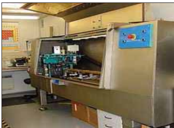
Figura 3.11. XRF core scanner (MARUM).
