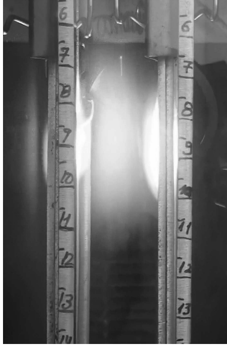
Figure 3.12: Image of one experiment. Case N = 2 , X_{O_2} = 30\% , and C = 28 mm.
