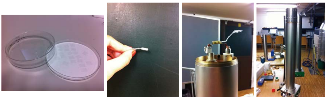
Figure 62: Preparation of samples for ssNMR. From left to right: (1) Sample preparation, (2) Sample wrapping (3) The samples are placed in the flat-coil probe and (4) The probe is introduced in the NMR spectrometer for the measurements.
