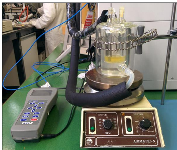
Figure 4.5. Equipment used for measuring solubility of salts in water at atmospheric pressure
