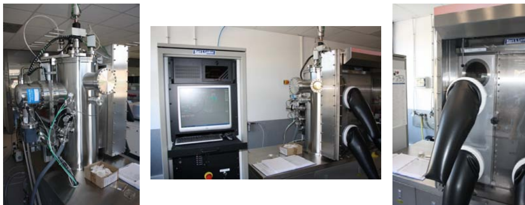
Figure 2.7. Back (left), lateral (middle) and front (right) views of the evaporation chamber attached to a glovebox.
