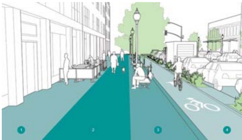
Fig. 1.7 Overview of a sidewalk. Numbers: 1 – frontage zone; 2 – pedestrian through zone; 3 – street furniture/curb zone; 4 – enhancement/buffer zone. Source: NACTO (2013).
